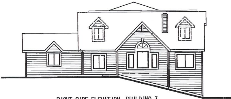
RIGHT SIDE ELEVATION BUILDING 3 SCALE 1/8" = 1'-0"
